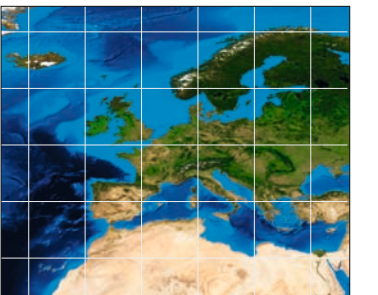
6a. In the geographic projection, the lines of constant latitude and longitude form straight lines.
