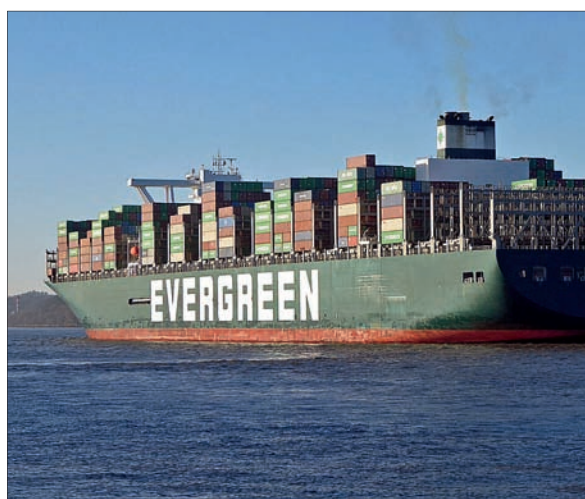
11. The Ever Given, a container vessel of the Evergreen shipping company. With its length of almost 400 metres it is one of the world's largest container ships and can transport more than 20,000 standard containers.
